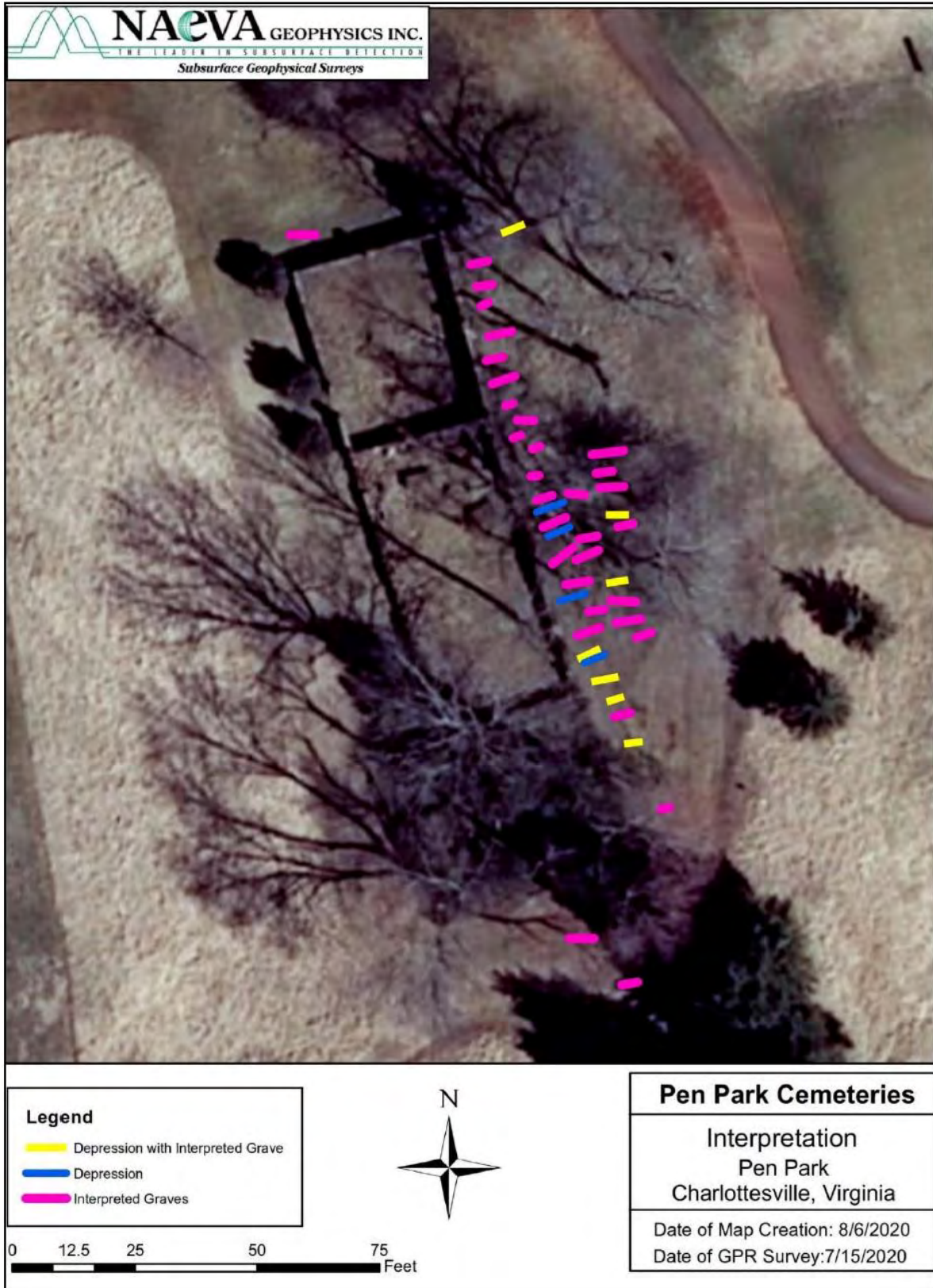
Pen Park cemetery and GPR identified potential grave shafts. (Fig. #15, RAS report.)
